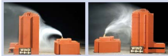
Figure 1a (left): Plume impact on taller downwind building. Figure 1b (right): Plume impact on taller upwind building.
