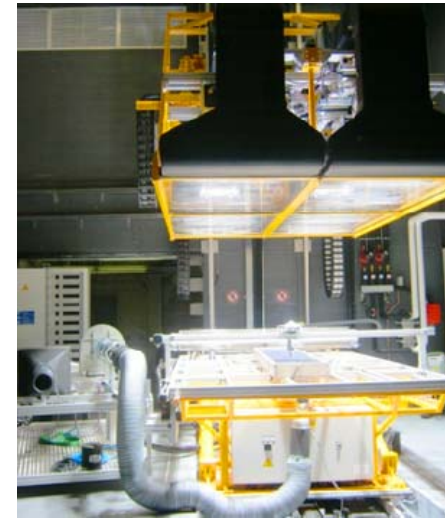
Concordia solar simulator testing BIPV/T system Roof system
